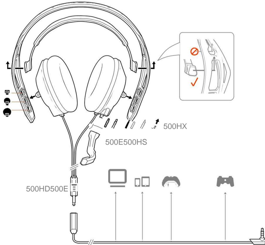
**TIP** When putting the sling and headband together, it is important to place the sling in the correct slot or it won't hold.
