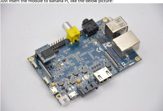
Just insert the module to Banana Pi, like the below picture:
