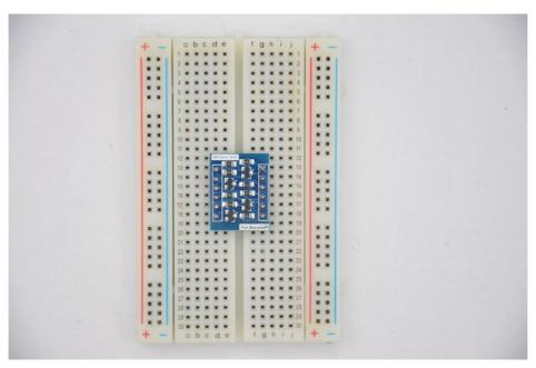
As show in picture, the left Header is the output or input port of lower electric level; The right Header is the output or input port of higher electric level.
