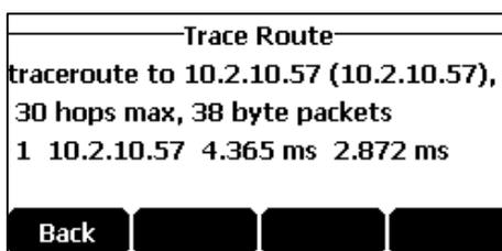
The first line of result is information about what you are doing. It shows the target, IP address of the target, the maximum number of hops that will be allowed, and the size of the packets being sent.
