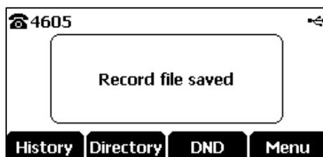
The recording will be stored as a new .wav file on the USB flash drive when the phone starts recording again.
