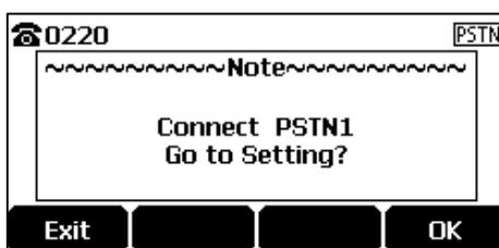
When two PSTN boxes are connected simultaneously to the phone successfully, the LCD screen prompts "Connect PSTN1 PSTN2 Go to Setting?".
