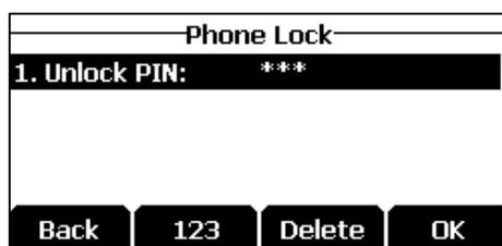
3. Tap the **OK** soft key to unlock the keypad.
