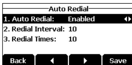
2. Enter the desired time (in seconds) in the **Redial Interval** field.
