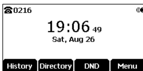
If the phone detects the USB flash drive successfully, the icon
