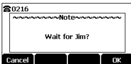
1. Tap the **OK** soft key, the phone returns to the idle screen and call completion is activated.
