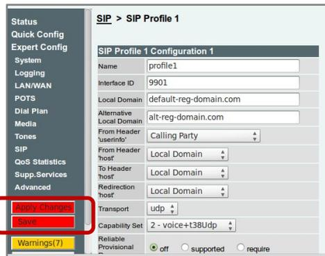
26. Once you have saved the changes, go to “Dial Plan” located on the “Expert Config” section (Figure 4.22)
