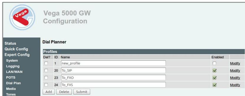
27. Here we’re going to create a dial plan to route the calls. Delete all the entries and create 3 profiles that will be used for incoming calls to FXS, FXO and SIP interface. Below is the configuration of each profile (Figure 4-23).
