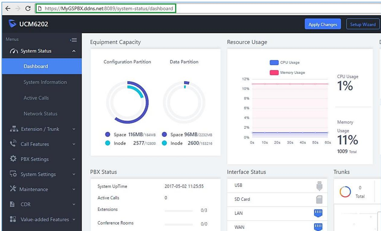
**Figure 27: Using Domain Name to Connect to UCM6200**
