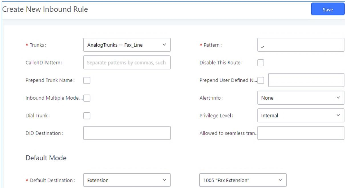
**Figure 164: Configure Inbound Rule for Fax**
