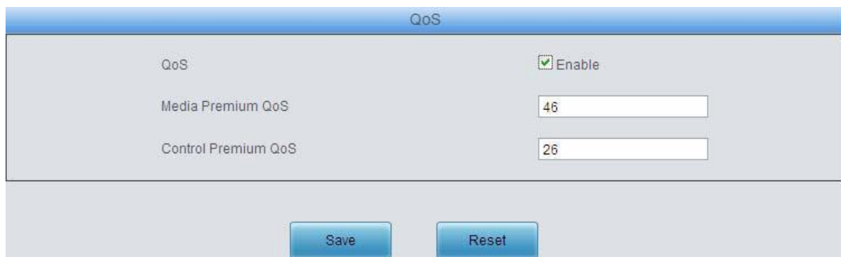
Figure 3-51 Differentiated Services Setting Interface
