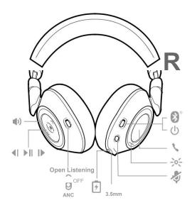
Volume Rotate the volume wheel **●**<sup>±</sup> forward (+) or backward (–) to control the volume.
