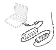
The USB adapter is automatically powered on upon inserting into the USB port of the computer.
