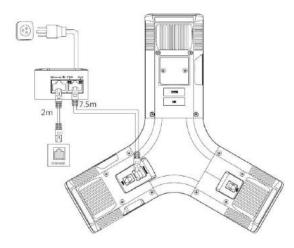
**Note** The IP phone should be used with Yealink original PoE adapter (54V/0.56A) only. The use of the third-party PoE adapter may cause the damage to the phone. The cable and wire should be replaced at once if its skin is broken.
