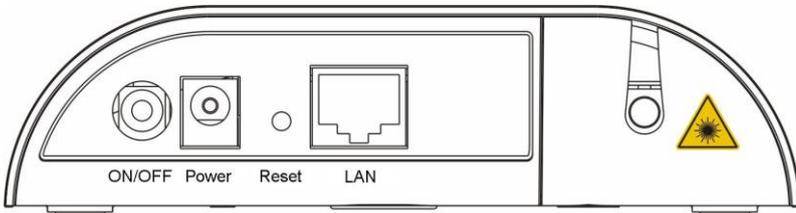
Figure 2-2 Front view of the AN5506-01-A rear panel
