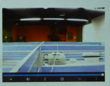
If the image display fuzzy is the lens focusing not properly, You can do a slight rotation of lens to do focal length adjustment, until the image become clearly
