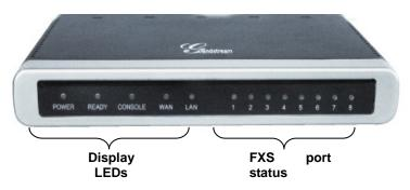
FIGURE 2: DIAGRAM OF GXW4004-8 DISPLAY PANEL
