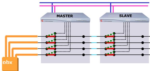
The status of the ISDN fallback relays can determine whether SIP registration takes place on a Vega E1T1 (models where ISDN fallback relays are fitted).
