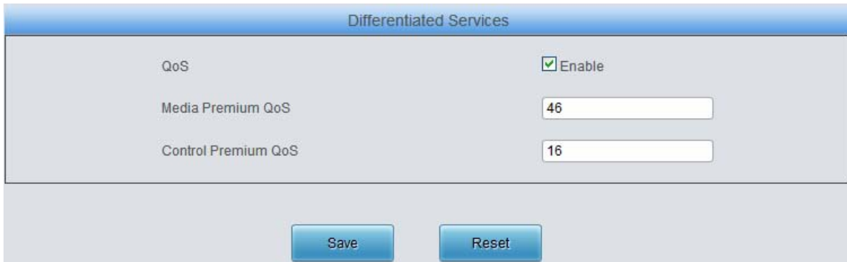
Figure 3-44 Differentiated Services Setting Interface
