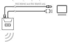
**IMPORTANT** Optical cable connection is only for RIG 800HD and RIG 800HS.
