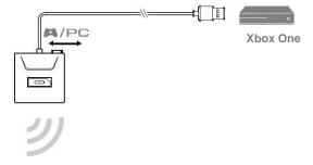
NOTE Ensure the switch on the back of the adapter is set to your preference: console or PC.
