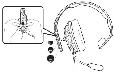
3 To position the microphone on the right or left side, rotate the microphone boom down and over.
